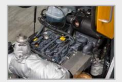
Maximum drive power thanks to the 44.5 kW Deutz engine – this meets all requirements of the current "Stage V" emission category.
